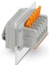
Panel feed-through terminal block, connection method: Push-lock connection, Push-in spring connection, number of positions: 5, load current: 41 A, cross section: 2.5 mm<sup>2</sup> - 10 mm<sup>2</sup>, connection direction of the conductor to plug-in direction: 0 °, width: 74.4 mm
