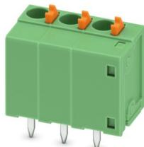
PCB terminal block, nominal current: 15 A, rated voltage (III/2): 400 V, nominal cross section: 1.5 mm<sup>2</sup>, number of potentials: 3, number of rows: 1, number of positions per row: 3, product range: FFKDS(A)/V2, pitch: 5.08 mm, connection method: Push-in spring connection, mounting: Wave soldering, conductor/PCB connection direction: 90 °, color: green, Pin layout: Linear pinning, Solder pin [P]: 3.4 mm, number of solder pins per potential: 2, type of packaging: packed in cardboard
