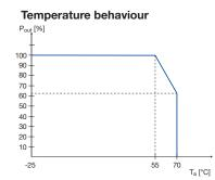
Temperature curve at rated load
