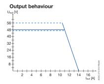
Output curve at  $T_a = 25 \text{ °C}$
