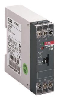
The CT-AWE is a single-function electronic time relay from the CT-E timer range. It provides an impulse-OFF (trailing edge interval) function with a time range from 0.1 s to 10 s. This time relay operates with a rated control supply voltage of 110 - 130 V AC and has a 1 c/o (SPDT) output rated at 250 V / 4 A. A control input works with voltage-related (non-floating) triggering.
