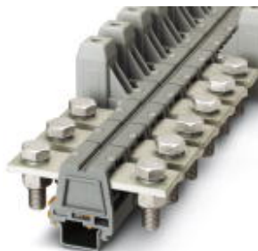
Universal terminal block with screw connection, cross section: 35 - 95 mm 2 , AWG: 2 - 4/0, width: 40 mm, color: gray
