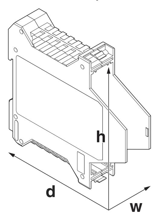
Schematic figure for illustrating the item dimensions. The figure is not of the desired product. For further details, refer to the product drawings in the "Downloads" tab.
