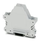
DIN rail housing, Lower housing part with metal foot catch, flat design, with vents, width: 22.6 mm, height: 99 mm, depth: 84.8 mm, color: light grey (similar RAL 7035), cross connection: integrated bus connector, number of positions cross connector: 10+2, Bus connector: 10 parallel contacts, 2 serial contacts
