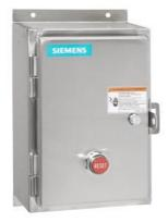
Reversing motor starter, Size 0, Single Phase, 2-Pole, Amb. compensate bimetal OLR, Contactor amp rating 18A, 110V 50Hz / 120V 60Hz coil, Non-combination type, Encl. type 4X 304 S. Steel, Water/dust tight noncorrosive
