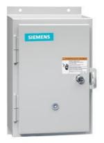
Reversing motor starter, Size 0, Three phase full voltage, Amb. compensate bimetal OLR, Contactor amp rating 18A, 208VAC 60Hz coil, Non-combination type, Enclosure type 12, Dust/drip proof for indoors
