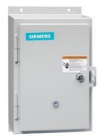
Reversing motor starter, Size 0, Three phase full voltage, Solid-state overload relay, OLR amp range 5.5-22A, 110V 50Hz / 120V 60Hz coil, Non-combination type, Enclosure type 12, Dust/drip proof for indoors, Standard width enclosure
