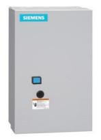
Reversing motor starter, Size 1, Single Phase, 2-Pole, Amb. compensate bimetal OLR, Contactor amp rating 27A, 208VAC 60Hz coil, Non-combination type, Enclosure type 1, Indoor general purpose use
