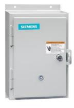
Reversing motor starter, Size 1, Three phase full voltage, Amb. compensate bimetal OLR, Contactor amp rating 27A, 208VAC 60Hz coil, Non-combination type, Enclosure type 12, Dust/drip proof for indoors
