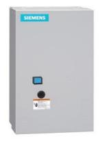
Reversing motor starter, Size 1, Three phase full voltage, Amb. compensate bimetal OLR, Contactor amp rating 27A, 24VAC 50-60Hz coil, Non-combination type, Enclosure type 1, Indoor general purpose use
