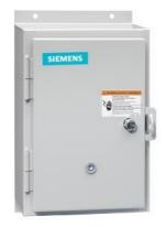
Reversing motor starter, Size 1, Three phase full voltage, Solid-state overload relay, OLR amp range 5.5-22A, 110V 50Hz / 120V 60Hz coil, Non-combination type, Enclosure type 12, Dust/drip proof for indoors, Standard width enclosure
