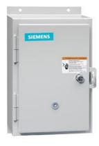
Reversing motor starter, Size 1, Three phase full voltage, Solid-state overload relay, OLR amp range 10-40A, 208VAC 60Hz coil, Non-combination type, Enclosure type 12, Dust/drip proof for indoors, Standard width enclosure
