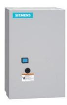
Reversing motor starter, Size 1 3/4, Single phase, 2-pole, Amb compensate bimetal OLrelay Contactor amp rating 40Amp 110V 50HZ / 120V 60HZ coil, Non-combination type, Enclosure type 1, Indoor general purpose use
