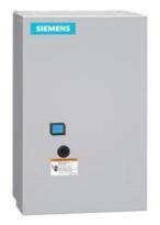
Reversing motor starter, Size 1 3/4, Three phase full voltage, Amb. compensate bimetal OLR, Contactor amp rating 40A, 208VAC 60Hz coil, Non-combination type, Enclosure type 1, Indoor general purpose use
