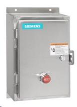
Reversing motor starter, Size 1 3/4, Three phase full voltage, Amb. compensate bimetal OLR, Contactor amp rating 40A, Non-combination type, Encl. type 4X 304 S. Steel, Water/dust tight noncorrosive
