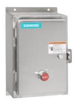
Reversing motor starter, Size 1 3/4, Three phase full voltage, Amb. compensate bimetal OLR, Contactor amp rating 40A, 110V 50Hz / 120V 60Hz coil, Noncombination type, Encl. type 4X 304 S. Steel, Water/dust tight noncorrosive
