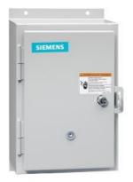
Reversing motor starter, Size 1 3/4, Three phase full voltage, Solid-state overload relay, OLR amp range 10-40A, Non-combination type, Enclosure type 12, Dust/drip proof for indoors, Standard width enclosure
