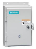
Reversing motor starter, Size 1 3/4, Three phase full voltage, Solid-state overload relay, OLR amp range 10-40A, 110V 50Hz / 120V 60Hz coil, Non-combination type, Enclosure type 12, Dust/drip proof for indoors, Standard width enclosure
