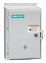
Reversing motor starter, Size 1 3/4, Three phase full voltage, Solid-state overload relay, OLRelay amp range 10-40a, 240V 50HZ / 277V 60HZ coil, Non-combination type, Enclosure type 12, Dust/drip proof for indoors, Standard width enclosure
