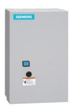
Reversing motor starter, Size 2, Three phase full voltage, Amb. compensate bimetal OLR, Contactor amp rating 45A, 110V 50Hz / 120V 60Hz coil, Non-combination type, Enclosure type 1, Indoor general purpose use
