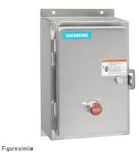
Reversing motor starter, Size 2, Three phase full voltage, Amb. compensate bimetal OLR, Contactor amp rating 45A, 24VAC 50-60Hz coil, Non-combination type, Encl. type 4X 304 S. Steel, Water/dust tight noncorrosive
