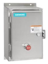
Reversing motor starter, Size 2 1/2, Three phase full voltage, Amb. compensate bimetal OLR, Contactor amp rating 60A, Non-combination type, Encl. type 4X 304 S. Steel, Water/dust tight noncorrosive
