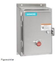
Reversing motor starter, Size 2 1/2, Three phase full voltage, Amb. compensate bimetal OLR, Contactor amp rating 60A, Non-combination type, Encl. type 4X 304 S. Steel, Water/dust tight noncorrosive
