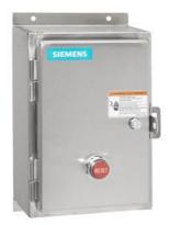
Reversing motor starter, Size 3, Three phase full voltage, Amb. compensate bimetal OLR, Contactor amp rating 90A, 208VAC 60Hz coil, Non-combination type, Encl. type 4X 304 S. Steel, Water/dust tight noncorrosive
