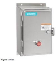
Reversing motor starter, Size 3, Three phase full voltage, Amb. compensate bimetal OLR, Contactor amp rating 90A, 24VAC 50-60Hz coil, Non-combination type, Encl. type 4X 304 S. Steel, Water/dust tight noncorrosive
