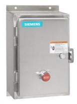
Reversing motor starter Size 3 Three phase full voltage Amb compensate bimetal OLrelay Contactor amp rating 90 AMP 240VAC 50HZ / 277VAC 60HZ coil Non-combination type Encl NEMA type 4X 304 S-steel Water/dust tight non-corrosive
