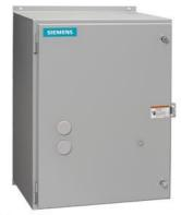
Reversing motor starter, Size 3, Three phase full voltage, Solid-state overload relay, OLR amp range 25-100A, Non-combination type, Enclosure type 12, Dust/drip proof for indoors, Standard width enclosure
