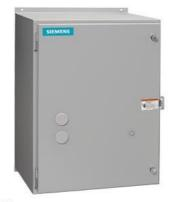
Reversing motor starter, Size 3 1/2, Three phase full voltage, Amb. compensate bimetal OLR, Contactor amp rating 115A, Non-combination type, Enclosure type 12, Dust/drip proof for indoors
