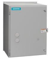
Reversing motor starter Size 3 1/2 Three phase full voltage Amb compensate bimetal OLrelay Contactor amp rating 115Amp 208VAC 60HZ coil Noncombination type Enclosure NEMA type 12 Dust/drip proof for indoors
