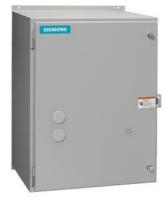
Reversing motor starter, Size 3 1/2, Three phase full voltage, Amb. compensate bimetal OLR, Contactor amp rating 115A, 110V 50Hz / 120V 60Hz coil, Noncombination type, Enclosure type 12, Dust/drip proof for indoors
