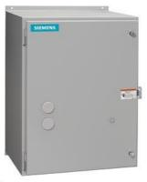
Reversing motor starter Size 3 1/2 Three phase full voltage Amb compensate bimetal OLrelay Contactor amp rating 115Amp 24VAC 50-60HZ coil Non-combination type Enclosure NEMA type 12 Dust/drip proof for indoors
