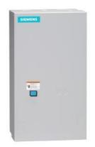
Reversing motor starter, Size 3 1/2, Three phase full voltage, Amb. compensate bimetal OLR, Contactor amp rating 115A, 110V 50Hz / 120V 60Hz coil, Noncombination type, Enclosure type 1, Indoor general purpose use
