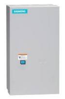
Reversing motor starter, Size 3 1/2, Three phase full voltage, Amb compensate bimetal OLrelay Contactor amp rating 115Amp 380 440/440 480V 50/60HZ coil, Non-combination type, Enclosure type 1, Indoor general purpose use
