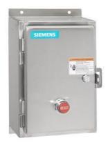
Reversing motor starter, Size 3 1/2, Three phase full voltage, Amb. compensate bimetal OLR, Contactor amp rating 115A, Non-combination type, Encl. type 4X 304 S. Steel, Water/dust tight noncorrosive
