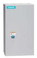
Reversing motor starter, Size 3 1/2, Three phase full voltage, Solid-state overload relay, OLR amp range 50-200A, 110V 50Hz / 120V 60Hz coil, Non-combination type, Enclosure type 1, Indoor general purpose use, Standard width enclosure
