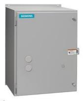
Reversing motor starter, Size 4, Three phase full voltage, Amb. compensate bimetal OLR, Contactor amp rating 135A, Non-combination type, Enclosure type 12, Dust/drip proof for indoors
