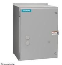
Reversing motor starter Size 4 Three phase full voltage Amb compensate bimetal OLrelay Contactor amp rating 135Amp 24VAC 50-60HZ coil Non-combination type Enclosure NEMA type 12 Dust/drip proof for indoors
