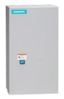
Reversing motor starter, Size 4, Three phase full voltage, Amb. compensate bimetal OLR, Contactor amp rating 135A, Non-combination type, Enclosure type 1, Indoor general purpose use
