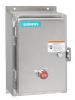
Reversing motor starter, Size 4, Three phase full voltage, Amb. compensate bimetal OLR, Contactor amp rating 135A, Non-combination type, Encl. type 4X 304 S. Steel, Water/dust tight noncorrosive
