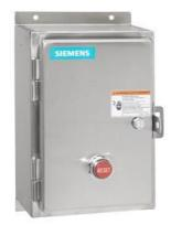
Reversing motor starter Size 4 Three phase full voltage Amb compensate bimetal OLrelay Contactor amp rating 135Amp 208VAC 60HZ coil Non-combination type Encl NEMA type 4X 304 S-steel Water/dust tight non-corrosive
