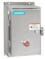
Reversing motor starter Size 4 Three phase full voltage Amb compensate bimetal OLrelay Contactor amp rating 135Amp Non-combination type Encl NEMA type 4X 304 S-steel Water/dust tight non-corrosive
