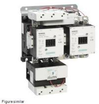
Reversing motor starter Size 5 Three phase full voltage Solid-state overload relay OLRelay amp range 55-250A 200-220V 50-60HZ/DC coil Non-combination type Enclosure type (open)
