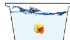
IP67: Submersion to one meter for 30 minutes.
