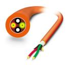
Robust GOF installation cable for assembly (IP20 heads only) for installation in stationary systems and machines, aramid strain-relief elements, with individual elements made from FRNC material, halogen-free, ozone and UV resistant, with a polyurethane (PUR) outer sheath
