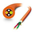
Fiber glass cable, duplex 50  $\mu m/125~\mu m,$  by the meter, without male connector, for installation in stationary systems and machines
