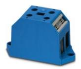
Device terminal block, Connection method: Screw connection, Number of connections: 4, Number of positions: 1, Cross section: 0.75 mm² - 35 mm², AWG: 18 - 2, Width: 34.8 mm, Height: 44.9 mm, Color: blue, Mounting type: Direct screw connection
