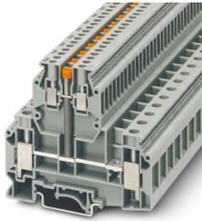
Double-level terminal block, with equipotential bonder, nom. voltage: 500 V, nominal current: 57 A, connection method: Screw connection, Rated cross section: 10 mm<sup>2</sup>, cross section: 0.5 mm<sup>2</sup> - 16 mm<sup>2</sup>, connection method: Screw connection, 2nd level, Rated cross section: 2.5 mm<sup>2</sup>, cross section: 0.2 mm<sup>2</sup> - 4 mm<sup>2</sup>, mounting type: NS 35/7,5, NS 35/15, NS 32, color: gray
