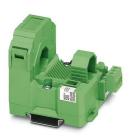
MCR current measuring transducer, for measuring sinusoidal and non-sinusoidal alternating currents, input current 0...100 A, loop-powered output with 4...20 mA
