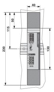
Mounting position: Installation depth 115 mm (+ DIN rail)
